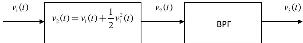
If the input signal  $v_1(t) = c(t) + m(t)$  is the sum of the carrier wave  $c(t) = \cos 8\pi f_m t$  and the message signal  $m(t) = \cos 2\pi f_m t$ ,
