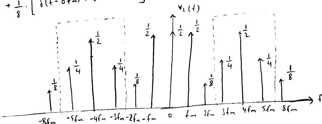
AM modulation signal =  $\underbrace{[1 + m \cdot \cos(2\pi f_m t)]}_{m(t)} \cdot \underbrace{\cos(8\pi f_m t)}_{c(t)}$
